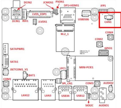
CANBus Connector (CAN1) on AIMB-U117 and EPC-U2117 PCBA
